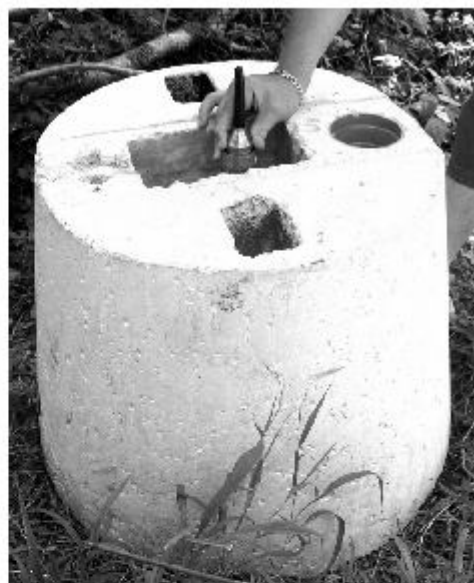
Fig. 2. Concrete block of 300 kg and its hydrophone.
